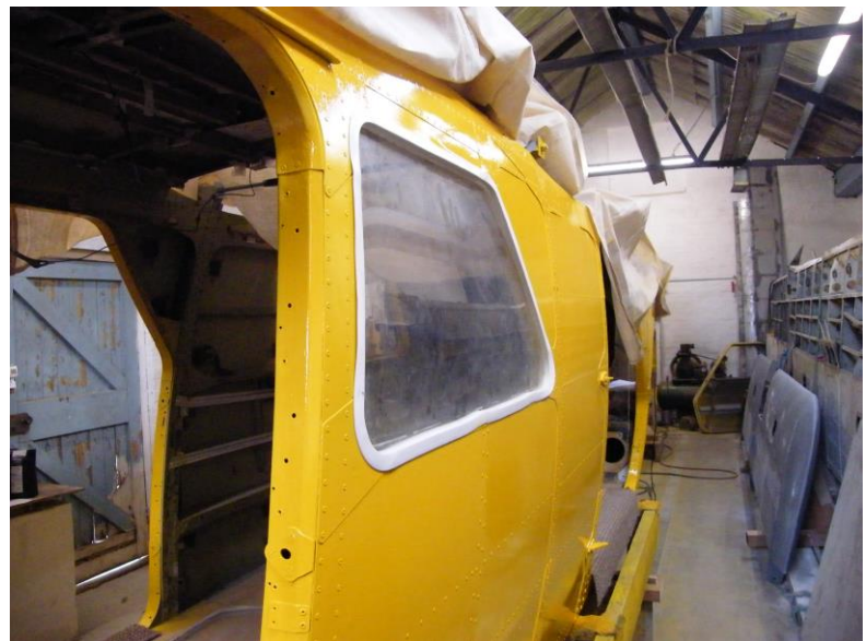
This port side passenger window was trial fitted using the recently purchased window mouldings
