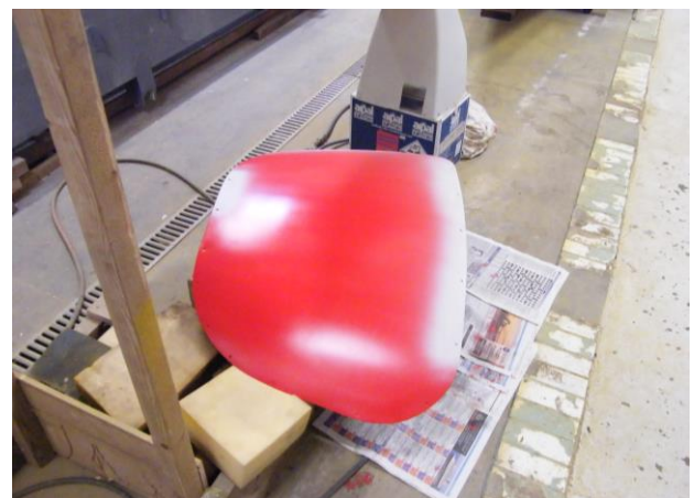
Avionics bay cover has been painted but needs to be re-painted after some blemishes became evident.
