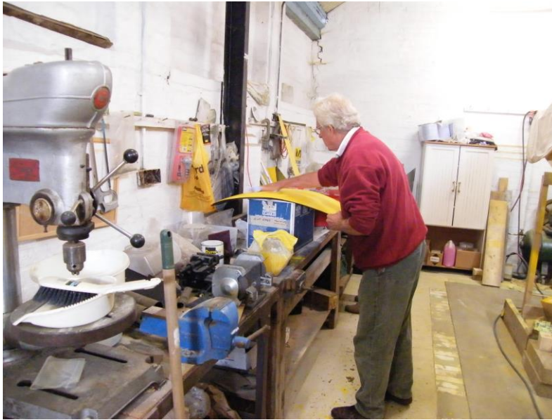
Bob Wilson reworking the surface of the avionics bay cover due to some blemishes becoming evident after the cover had been painted.
