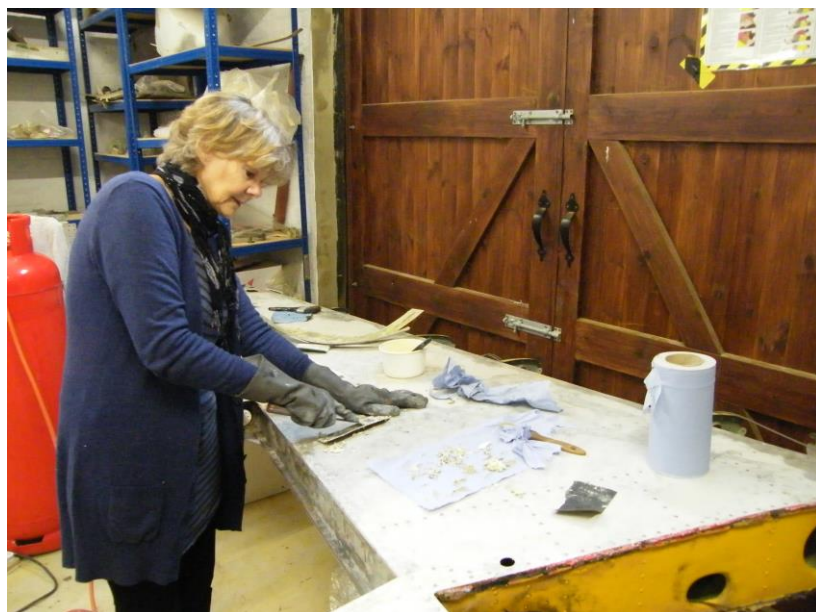
Rita Edgcombe returned to paint stripping the fin and preparing the external surfaces for etch priming.
