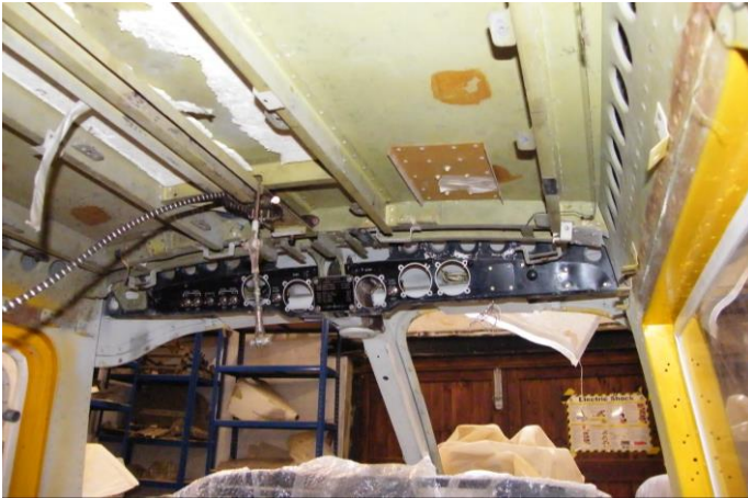
Interior view showing the "Eyebrow" panels after installation.
