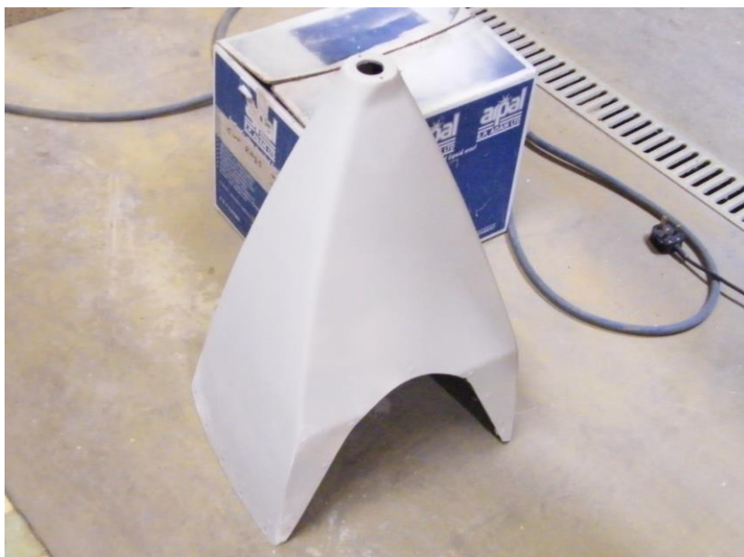
Tail cone is shown here after repair and priming ready for top coat painting.
