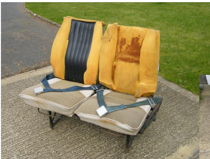
Seat back covers are missing and seat cushions are well worn and not considered re-usable.
