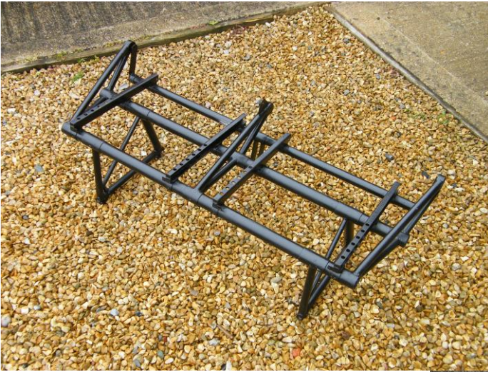
Pilot's seat main support frame after refurbishment by Andy Stewart.
