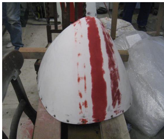
The fibreglass nose cone was in sound, relatively undamaged condition and has been sanded down ready for painting.
